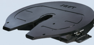
JSK54 Imposed Load: 80 t D Value: 550 kN Heavy Duty Fifth Wheel – 4"
