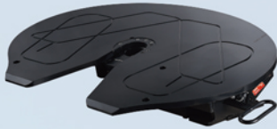
JSK52 Imposed Load: 74 t D Value: 400 kN Heavy Duty Fifth Wheel
