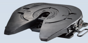
JSK50 Imposed Load: 50 t D Value: 300 kN Heavy Duty Fifth Wheel
